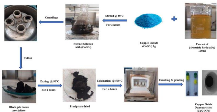
Figure 3: Diagram illustrating the protocol for preparing CuO NPs by leaf extract of ( Artemisia alba herba ).
