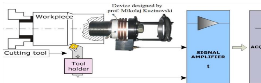
Figure 5. Working environment for the exploration of the average temperature in the cutting process during turning, using a computerized measurement system.
