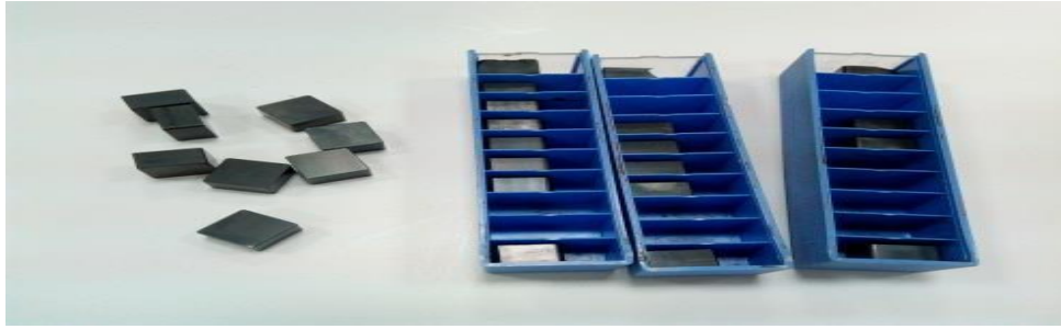
Figure 4. Cutting insert SNGN 120708-120712-120716 from mixed ceramics MC 2 (Al 2 O 3 + TiC) from the company HERTEL.
