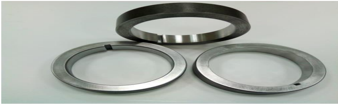
Figure 1. Rings of material C 50 (DIN), with hardness 50 \pm 2 HRC
