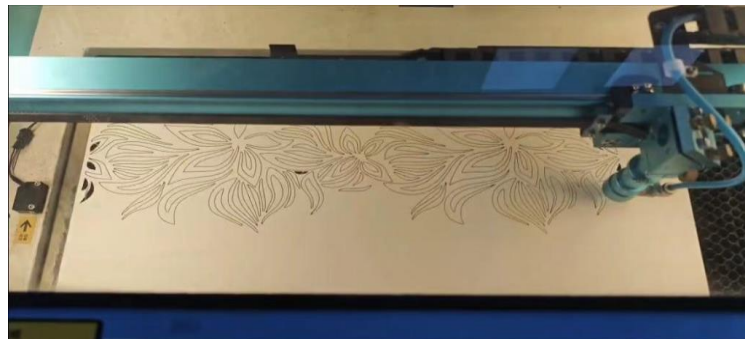
Figure 9: Stencil made by laser engraving
