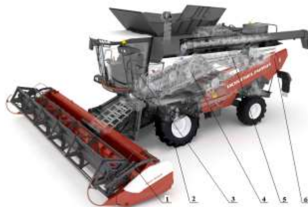
Figure 2: Process diagram of the RSM-181 TORUM-740 combine harvester (units: 1 – harvesting unit; 2 – running gear; 3 – controls; 4 – threshing unit; 5 – engine unit; 6 – chopper)
