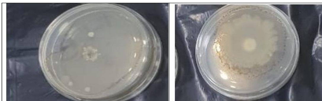
Figure 1: The formation of clear zone as result to degrade asphalt by bacterial isolate A8 that appeared the highest diameter of clear zone (27 mm) on MSM agar (Latha and Kalaivani ,2012). Demonstrated that on mineral salt media, the largest clearance zone was formed by two bacterial isolates. On the seventh day of incubation, S2 ( Bacillus subtilis ) among these isolates displayed the highest growth (0.85 mg/ml) and degradation, followed by S10 ( Pseudomonas aeruginosa ) (0.92 mg/ml). By using the plate assay method, the capacity of different bacterial strains to degrade asphalt was examined. Pseudomonas aeruginosa (27 mm in diameter) had the highest zone of exhibition in this investigation compared to Bacillus cereus (6 mm in diameter) (Sahu et al .,2019).
