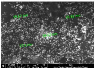
Figure 7: SEM image of AgPFNPs formed by P. farcta fruit extract. Scale bar: 1 μm Hemocompatibility assessment of AgPFNPs
