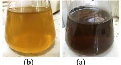
Figure 3: Eco-friendly AgPFNPs nanoparticle fabrication (a) Time 0 of (Prosopis. farcta + AgNO<sub>3</sub>) aqueous solutions incubation, and (b) 60 min post AgNPs fabrication
