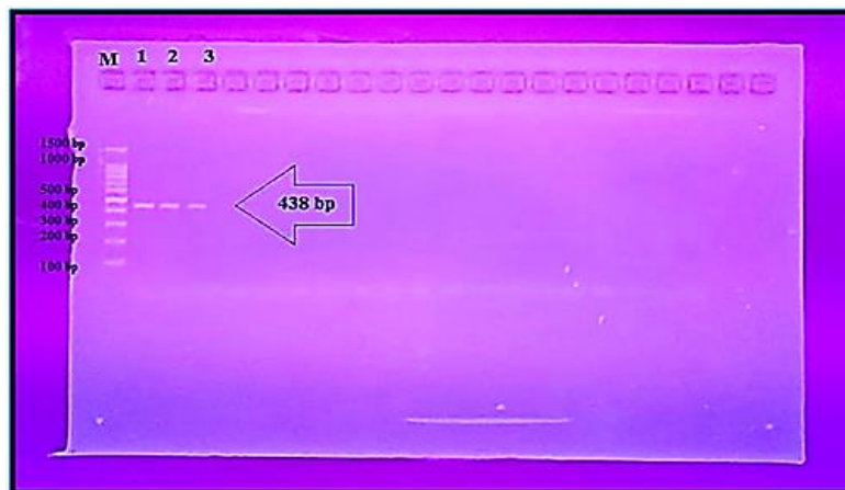
Figure (5): Identification of BLA- OXA 48 gene: the PCR product at band size 438bp. (Lane M:100 bp DNA marker, Lane 1-3 represent BLA- OXA
