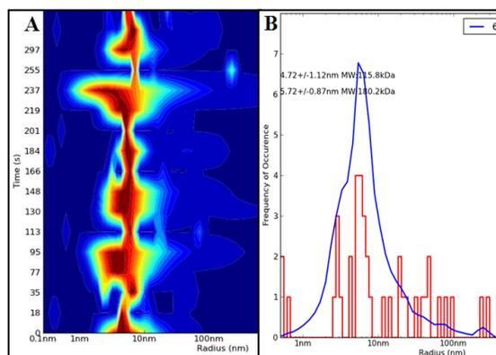
**Fig. 4: Dynamic light scattering (DLS) measurements of the purified globulin. (A) Purified CsCr dissolved in 25 mM phosphate buffer (pH 7.0) showed a monodispersity of oligomeric form of a 50 kDa monomer. (B) A monodisperse stable protein solution with a hydrodynamic radius (R<sub>H</sub>) of approximately 5.72 nm indicating the presence of trimeric (~180 kDa) nature.**
